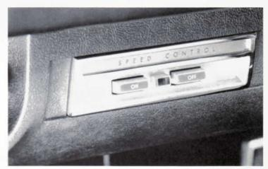
A Speed Control automatically maintains the desired speed, while permitting free movement of the feet for greater comfort on the highway. Stepping on the brake—or pressing the OFF button—shuts off the Speed Control device.
