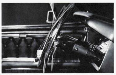
The Optional Tilt Steering Wheel, which adjusts up or down to any of nine positions, permits the driver to position the wheel at the angle most comfortable for him.
