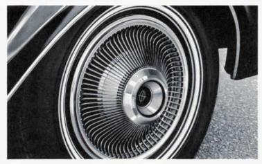
Owners may choose either single or dual chamber, fiber-glass belted, triple-band, white sidewall tires. The dual chamber retains air even in the event of a blowout.
