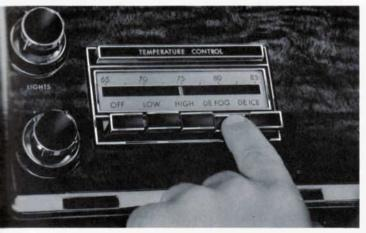
Continental's superior Air Conditioning is a big comfort option that's considered more of a necessity than a luxury these days. Available in either a manual control or Automatic Temperature Control system, the Continental air-conditioner cools, dehumidifies and filters air.
