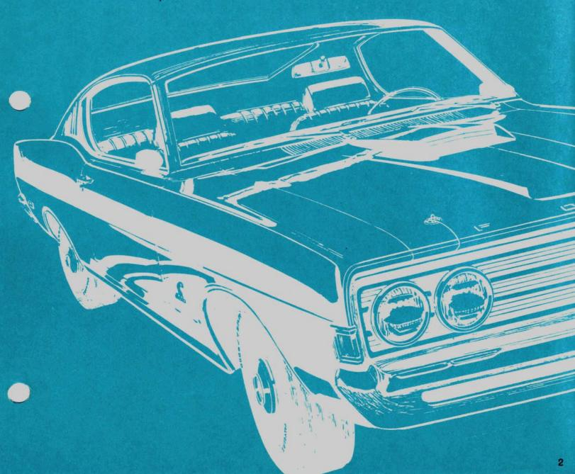
The Cobra's standard competition suspension is just what performance prospects want. It's beefed up for minimum body roll and maximum directional stability. It has high-rate front and rear springs, a large diameter front stabilizer bar, and high damping shocks for the best combination of performance ride and handling.
