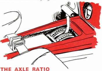
From the transmission, engine torque is carried by the driveshaft to the driving axle or differential, where it goes through another multiplication before it gets to the wheels. Axle ratios run from about two-point-seven to one on street machines with automatic transmissions to as high as six-and-one-third to one on competition cars. A numerically high ratio means better acceleration; while a lower ratio lets the engine turn at lower R.P.M.'s and often gives a higher top speed in miles per hour.
