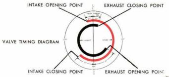
High duration and overlap are fine for developing more power at high speed, but cause loss of power and rough operation at low R.P.M.
