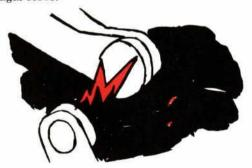
Ignition advance means that the spark is timed to make its mighty leap *ahead* of top-dead-center on the compression stroke. The spark *leads* the piston somewhat as you lead a bird with your 12-gauge shotgun; so that the gases a already starting to burn as the piston passes over center. The faster the engine goes, the more advance is needed, because there is a time lag between sparking and complete combustion.
