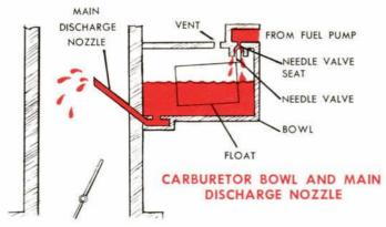
One way to get a *richer* mixture to the cylinders is to bend a little tang on the inlet valve float in the carburetor so as to raise the level of fuel in the bowl.
