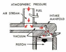
The *intake manifold* is a cast chunk of ductwork used to get the mixture from the carburetor to the intake ports in the cylinder head. There, the mixture is allowed to flow ito the individual combustion chamber when the *intake valve* opens. The burnt gases are pushed out or scavenged through the *exhaust valve* on the exhaust stroke of the piston.
