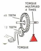
The drive train, besides transmitting power to the driving wheels, also has to multiply engine torque. The first place that torque multiplication happens is in the transmission; and it happens the most in the lowest gear. How much is torque multiplied? Depends on the gear ratio; which is equal to the number of teeth in the driven gear divided by the number of teeth in the gear that does the driving.
