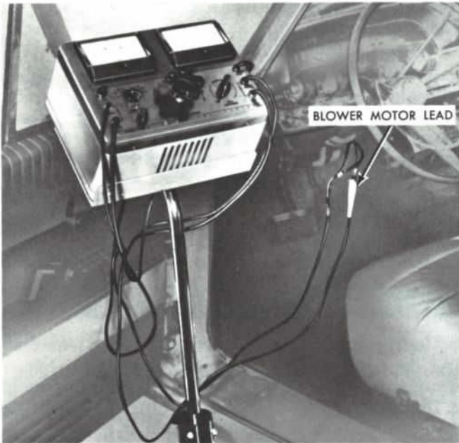
Fig. 21 — Blower Current Draw Test
