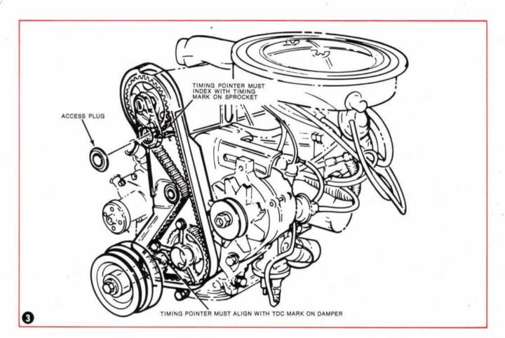
Now, remove the drive belt and inspect it for wear or visible damage. Replace if necessary. Position the crankshaft sprocket, the camshaft sprocket and the auxiliary shaft sprocket as shown in Figure 3.
