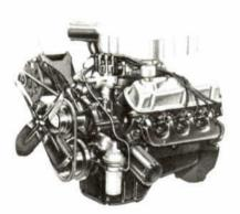
This engine is a new offering for the Mustang and Fairlane. With its rating of 225 horsepower it provides an ideal power option between the base 289 and the high performance 289 CID engine. The 289 4-V is identical to the base 289 V-8 except for the 4-venturi carburetor, increased compression ratio, dual exhaust system, different valve timing and the use of premium grade fuel.
