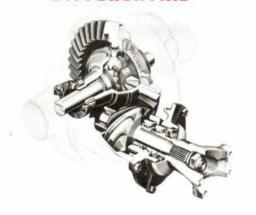
The optional limited-slip differential is available with all engines except the "427" High-Performance engine in the Ford line. If there are uneven traction conditions, the built-in clutch plates in the differential transfer part of the usable driveshaft torque to the wheel with the better traction. Thus, the car is much more likely to get under way because the usable traction is fully utilized.
