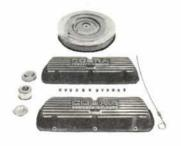
PART NUMBERS C40Z-6980-A C40Z-6A547-A } —260-289 C.I.D. Engines
