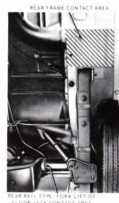
Figure 4— Hoisting the Mustang Rear Contact Areas
