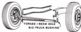
Forged steel I-beam axle attaches wheel to frame, locks in wheel camber. Axle pivots in husky, chatter-proof bushing.
