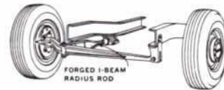
Big-truck radius rod secures axle to frame side rail. Stabilizes front end, locks in wheel caster.
