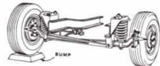
Each front wheel—on its own axle—operates independently to smooth the ride on the roughest roads.
