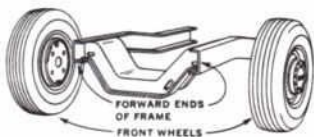
Object: Suspend front wheels independently, yet retain big-truck durability of solid I-beam axles.
