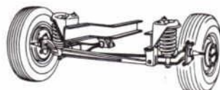
Opposite wheel is similarly suspended. Each wheel has its own forged steel I-beam axle, radius rod and spring.
