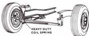
Heavy-duty, non-sag coil spring gives entire suspension low-friction, easy-riding action.
