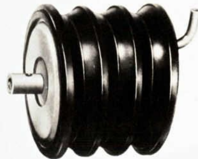
Figure 5—Vacuum Servo—mounted on a bracket under the instrument panel on the brake pedal support. The servo is linked to the carburetor throttle shaft. The links are held on by the use of snap rings.
