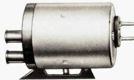
Figure 4—Vacuum Valve—mounted on the left-hand fender well. It is connected by vacuum hoses to the metering valve and car vacuum.
